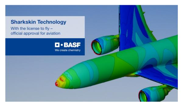
Lufthansa Technik is using CFD simulations to determine how drag is reduced by means of the bionic riblet film, among other things. These provide important results, not only for the design of the pattern. This is because before an aircraft type modified with sharkskin is allowed to transport passengers or goods through the air, it needs aviation authority approvals.
