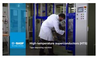
The superconductor bands are manufactured in several manufacturing steps. To ensure that the tape runs in the same direction during each step and that the same end of the tape can be processed first in each step, the tape is respooled.
