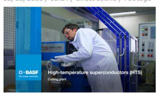
Once all coating processes have been completed, the tape is cut to the customer-specific width using cutting rollers.
