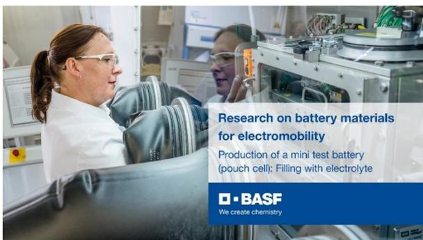
To gain insights into the properties of cathode materials produced in the laboratory, BASF researchers use pouch cells. Pouch cells are a common cell type in electric vehicles with a lithium-ion battery. A few hundreds of such cells are assembled therein.
